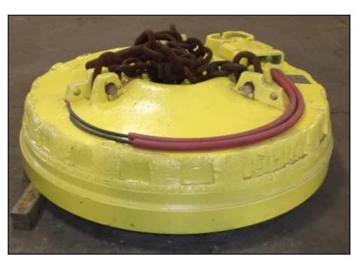
Size: 71" Type: **DAWX** Volts: 230 DC 104.5 Amps: Ohms: 2.2 Manufacturer: Ohio 9,150 lbs Weight: Duty Cycle: 75%
